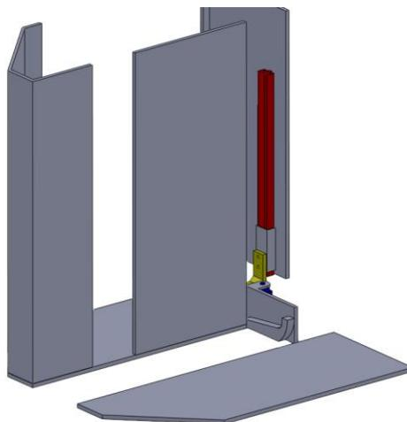
**Fig. 4.** Corn collecting mechanism. Door for precise positioning.
